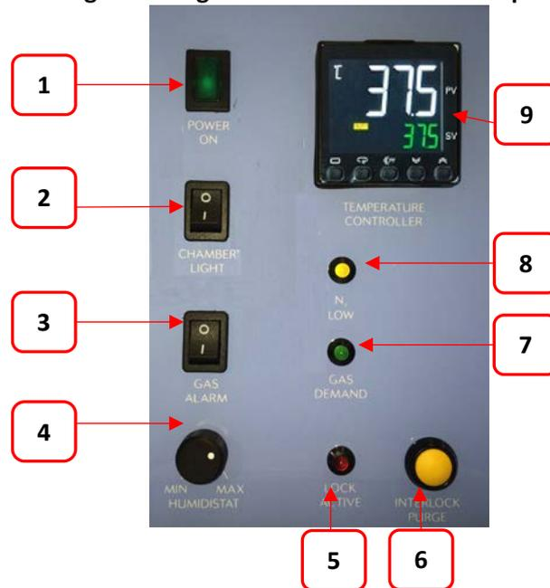
1. Power indicator. Illuminates to indicate the workstation is connected to the mains and is switched on.
